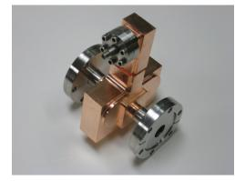
Beam Quadrupole Monitor
