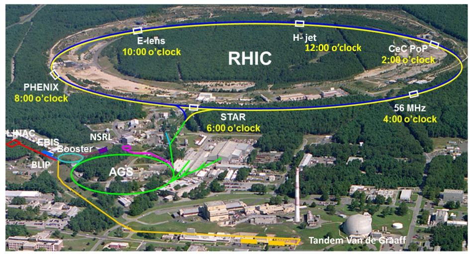
Brookhaven National Laboratory (BNL) Relativistic Heavy Ion Collider (RHIC) NASA Space Radiation Laboratory (NSRL) Linac Isotope Production (BLIP) / Medical Isotope Research and Production Program Tandem van de Graaff accelerators
