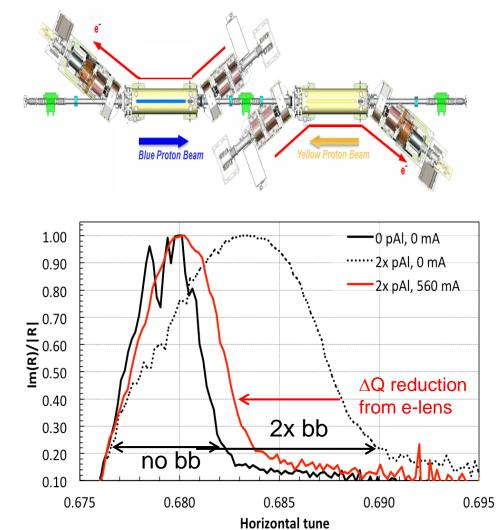
W. Fischer et al, Operational head-on beam-beam compensation with electron lenses in the Relativistic Heavy Ion Collider,
