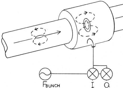
Determination of the beams Polarization and/or Magnetization by measurement of the phase and amplitude of the TE011 resonance induced.
