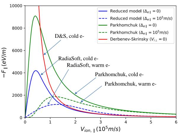
Param's are taken from Fedotov, Bruhwiler *et al.*:  $Au^{+79}$ ;  $\gamma = 107$ ;  $n_e = 10^{15} m^{-3}$ ; B = 5 T  $\tau_{int} = 4x10^{-10} s \sim 56 T_{Larmor} \sim 0.16 T_{plasma}$  $typical e^{-} sep. \sim 4.9x10^{-6} m \sim 10 r_{Larmor}$
