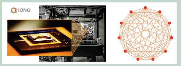
Figure 1: lonQ's trapped-ion digital quantum computer. The left panel shows the quantum computer along with an enlarged view of the ion trap (produced by SNL). The right panel shows the (all-to-all) connectivity map of the 11-qubit QC trapped ion systems that lonQ recently benchmarked. | *Images reproduced with permission from lonQ, via Jungsang Kim of Duke University*.
