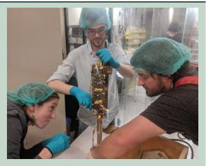
Figure 1: ADMX personnel assemble a cryo-electronics package containing a JPA and a TWPA for their axion search. | *Image reproduced with permission from Gray Rybka, University of Washington.*
