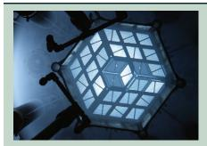
Figure 3: The MIT reactor being used to produce <sup>64</sup>Cu for use in controlled background experiments to measure the impact of radioactivity on quasi-particle distributions in superconducting qubits. | Image reproduced with permission from Joseph Formaggio, MIT.
