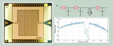
Figure 2: (a) A micrograph of a TWPA showing the path of traveling waves. (b) RF schematic for Josephson TWPAs. (c) Experimentally measured gains of a Josephson TWPA showing wideband performance. | Images reproduced with permission from William Oliver, Massachusetts Institute of Technology, Lincoln Laboratory.
