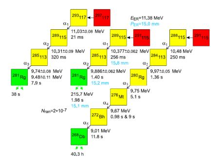
Decay properties of Z=117 and Z=115 isotopes averaged over observed five <sup>293</sup>(117) chains and twenty four <sup>288</sup>(115) chains [1]. The decay pattern of directly produced <sup>289</sup>(115) isotope provides an additional evidence for the recent identification of 293(117) nucleus [2].
