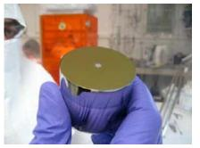
Germanium detector and the cryostat for Majorana Demonstrator.
