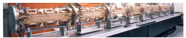
Figure 3: The LEDA RFQ without any of the umbilicals attached to the exterior. The 8 meter long accelerator is comprised of four 2 meter long sections. The cavity uses approximately 2 MW of power when operating, dissipating most of the energy into heat taken out by the cooling system (17).
