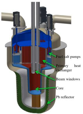
Figure 1. ADS molten salt core assembly.
