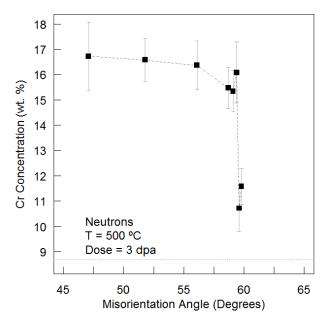
Figure 33: On-boundary Cr concentration in Fe-9%Cr binary alloy as a function of misorientation for high angle grain boundaries near the S2 origin
