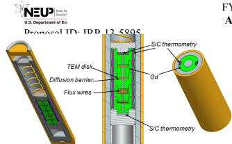
Figure 16: HFIR Irradiation Capsule Design for a Previous Texas A&M University Fast Neutron Irradiation
