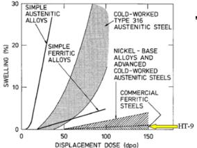
Figure 29: Swelling comparisons between HT-9 and other potential cladding materials.
