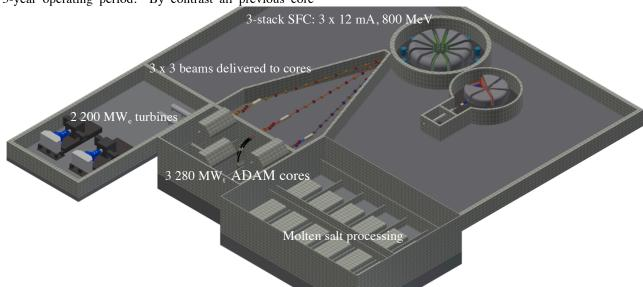
Figure 8.3-core ADAM facility that destroys transuranics at the same rate they are produced by a  $GW_e$  nuclear power
