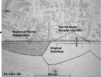
Figure 25: As-HIPed diffusion couple of the FGC, 100x (<u>39</u>)
