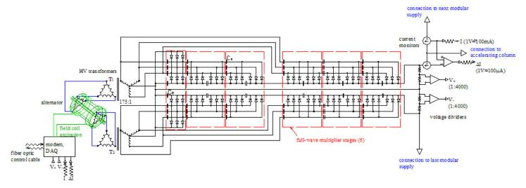
FIGURE 2. Circuit of one CMA module.
