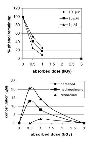
**FIGURE 6.** Simulation of electron beam treatment of phenol in water as a function of dose, from Ref. 5 : a) destruction of phenol; b) appearance and destruction of intermediaries.
