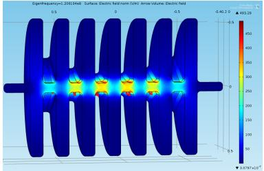
Figure 12: First iteration of the 6 cell kicker for the separation strategy. This cavity can provide 2 degrees of deflecthe same eccentricities during operation.
