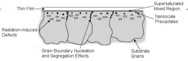
Figure 30: Types of irradiation damage at near interface area
