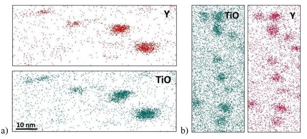
Figure 35: Atomic probe tomography (APT) elemental maps of the (a) as-received (unirradiated) 9%Cr ODS and (b) neutron irradiated 9%Cr ODS to 3 dna at 500°C showing
