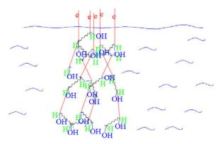
FIGURE 7. Ionization cascade in water makes free radicals.
