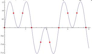
Figure 11: The spectrometer system uses two cavities operating at 58.3 MHz and another at 175 MHz to either increase or decrease the energy to allow different trajectories for 3 beams in the uniform magnetic field. The graph is an overlay of the two modes with the bunches indicated in red. The three beams (+,-,0) all have two bunches each. A single cavity (58.3 MHz) could be used if the particle speed were higher
