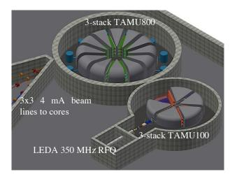
Figure 4. Acceleration chain for an ADAM site.
