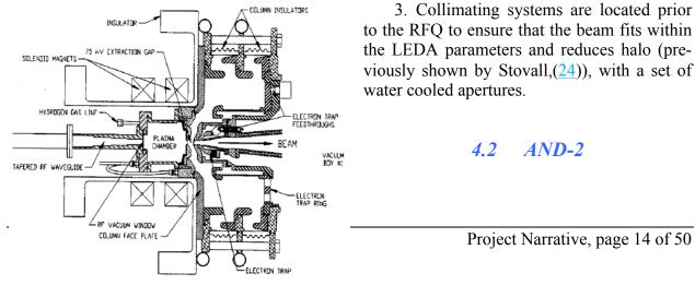
June 9, 2014 Figure 10: LEDA target as designed by CLR for the Chalk River Injector Test Stand (20).
