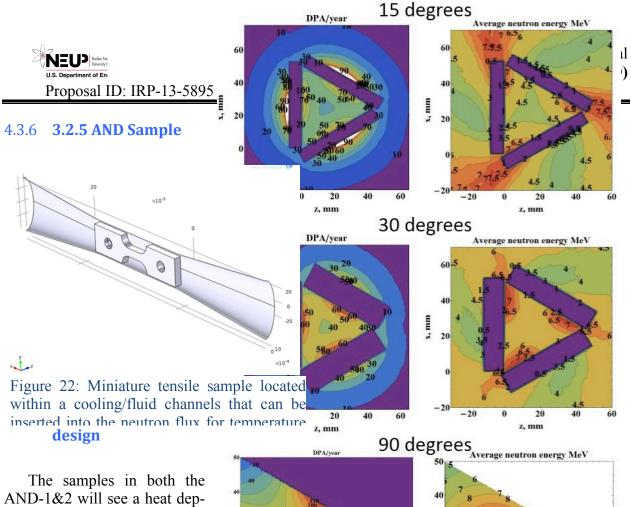
AND-1&2 will see a heat deposition. As consequence, the samples need to be cooled. Investigating the most extreme scenario for sample heating, the heat deposition in AND-2, at a strategy was devised to maintain the sample at a specified temperature. Samples at max DPA zone will receive up to 100W/cc, so helium gas cooling as possible way to control sample temperature was modeled. A heat load of 100 W/cc was applied to standard tensile specimen made
