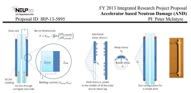
Figure 31: Proposed test schemes for SiC/SiC cladding tube and joint using a surrogate core tube; (right) a Nernst glower bar: L=45mm, dia=2.7 mm in dia.
