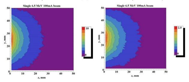
Figure 19: Left: The DPA received by a nickel sample bathed in the neutron flux, generated by the 6.5 MeV protons, directly behind the Lithium target. Right: Heat generated by the beam in  $\varphi(E)$  then is given as
