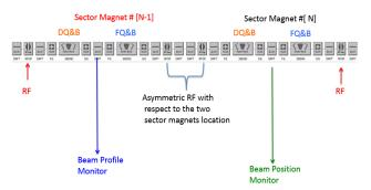
Figure 2. Lattice elements in the tracking simulation of one cell (sector dipoles) of the SFC lattice.
