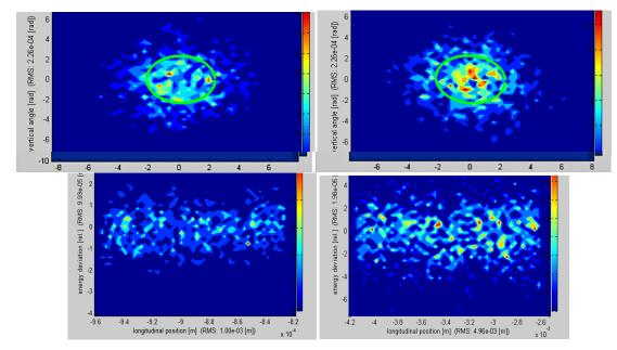
Figure 6. a) Beam breakup in transverse phase space after  $2^{nd}$  orbit when tune is near  $3^{rd}$  order and  $5^{th}$ -order resonances; b) beam breakup in longitudinal phase space when tune is near  $5^{th}$  order resonance.
