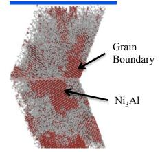
Figure 37: Monte Carlo simulation of  $Ni_3Al$  precipitation, next to a grain boundary in a Ni-0.10at.Al at 900K.
