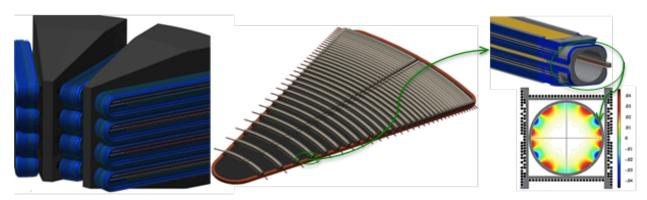
Figure 13: Left Superconducting cavities in blue. Middle: a sector magnet with a FODO lattice of quad focusing channels which tightly control the beam to allow high current. Right: close up of Quad and magnetic field cross section.
