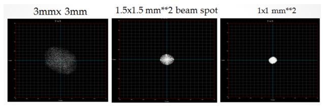
Figure 7: TRACE 3D simulations for the beam from the source to the LEBT. The accelerator group optimized the solenoid settings of Trace-3D such that the output of the simulation provides the design value given by LANL scientists during design and commissioning of the LEDA.
