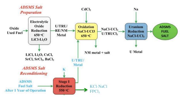
Figure 2. Pyroprocessing and electro-separation processes used to prepare the fuel salt.
