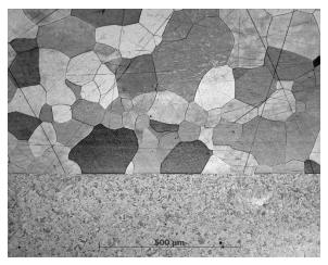
Figure 28: Micrograph of the as manufactured FGC, 100x. Irradiation induced mixing is a kev concern for the FGC (39).
