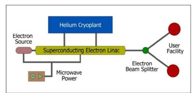
Figure 2. Conceptual Layout of the Niowave Superconducting Electron Linac used for various applications
