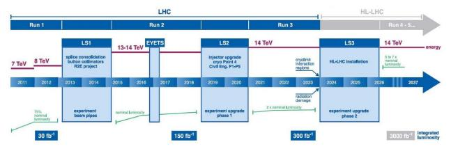
Figure 1: Operations, Upgrade, and Installation schedule for the Large Hadron Collider and the LHC Experiments, including the planned timeline for long shutdowns of the LHC, the center-of-mass energy and integrated luminosity during past and anticipated future physics runs. The nominal luminosity is the LHC design at  $1 \times 10^{34}$  cm<sup>-2</sup>s<sup>-1</sup>. Dates indicate calendar year.
