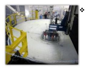
Fabrication of M1/M3 mirrors: final abrasive grinding, then polishing – complete by end of CY2012
