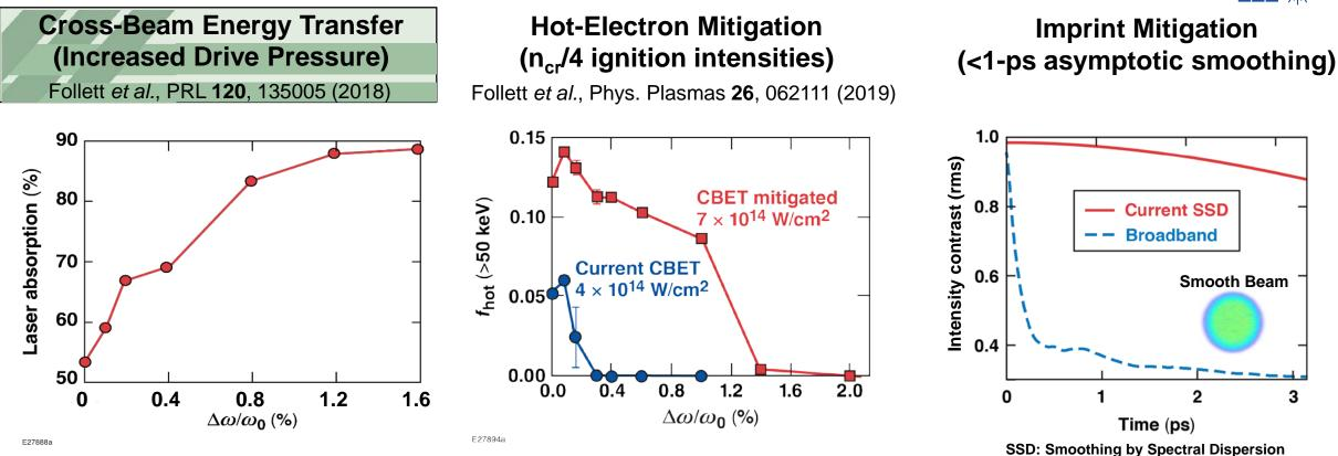
Laser bandwidth  $\Delta \omega/\omega > 1.5\%$  is predicted to mitigate hot electron generation, increase the laser absorption, and eliminate imprint, which will enable a robust ICF implosion
