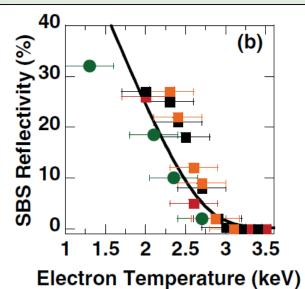
Higher temperature plasmas (>3 keV) are required for efficient laser beam propagation in hohlraums
