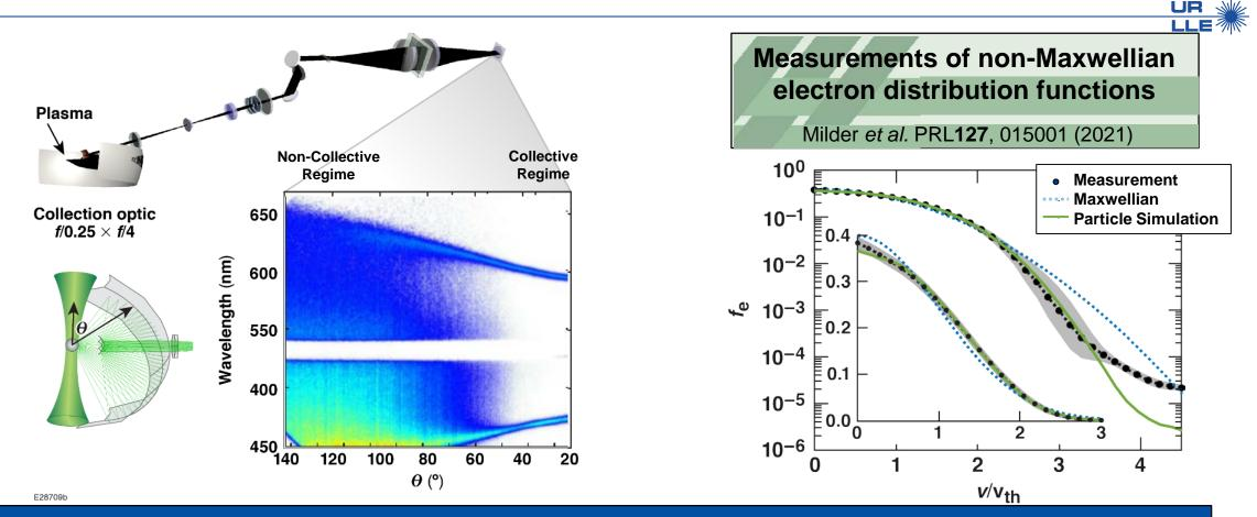
Measuring the plasma conditions is enabling the hydrodynamic uncertainties to be decoupled from the laser-plasma instability physics opening the design space for grand challenge applications
