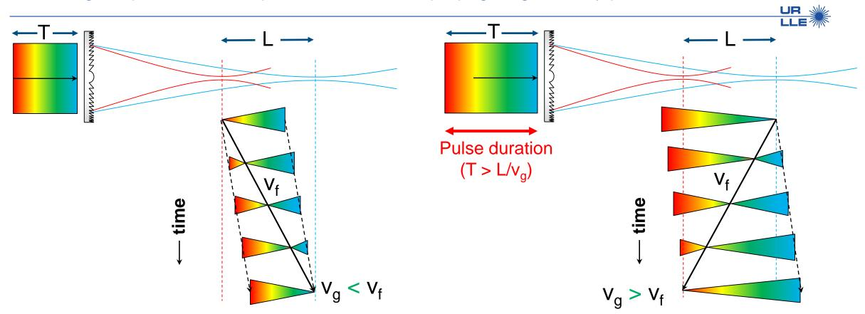
The chromatic focusing creates an extended focal range, while the chirp sets the time at which each frequency comes to its focus providing control over the velocity of the intensity peak
