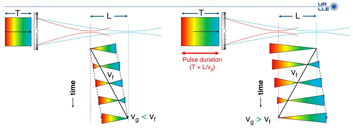
The intensity peak is propagating faster than the group velocity of light
