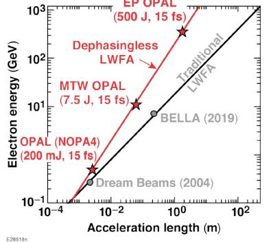
Spatiotemporal pulse shaping provides the opportunity to accelerate electrons to TeV energies in few-meter single-stage plasma without the need for a guiding structure
