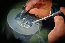
Cryo-electron microscopes, such as the one shown here, are the most powerful in the world because they capture images with electrons, not light. Samples are frozen in a super-cooled container (inset). (CREDIT: LAWRENCE BERKELEY NATIONAL LABORATORY)
