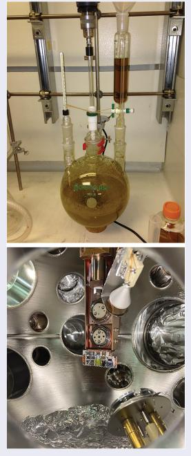
(Top) The chemical reactor set-up Colin Wessels used at the Molecular Foundry for making Prussian blue materials, with a synthesis in progress (CREDIT: NATRON ENERGY)
