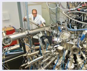
Ivan Bozovic with the atomic-layer-by-layer synthesis system he developed and uses at Brookhaven National Lab to engineer superconducting materials one atomic layer at a time. (CREDIT: BROOKHAVEN NATIONAL LABORATORY)
