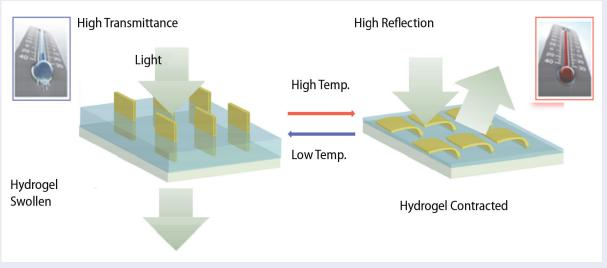
Schematic showing the mechanism by which temperature-sensitive hydrogel polymers can self-regulate the transparency of window (CREDIT:DR. PHILSEOK KIM, AIZENBERG LAB)
