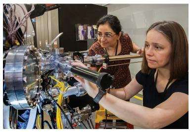
A Brookhaven National Laboratory staff scientist and a visiting researcher mount a material sample to measure its electronic structure with the laboratory's X-ray synchrotron. (CREDIT: BROOKHAVEN NATIONAL LABORATORY)
