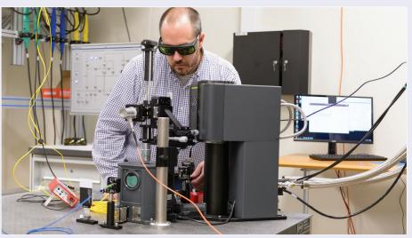
Argonne scientist Alan Dibos aligns optics to study materials for a possible quantum repeater device; the materials are in a cryostat that that keeps them at a temperature just 3 degrees above absolute zero. (CREDIT: ARGONNE NATIONAL LABORATORY)
