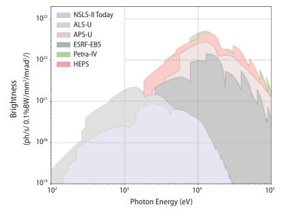
FIGURE 5. Brightness of U.S. synchrotron sources NSLS-II, ALS-U and APS-U compared with ESRF-EBS (France), Petra-IV (Germany) and HEPS (China)
