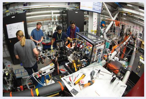
The experimental setup for documenting the chemistry of the water-splitting reaction at the XFEL X-ray laser (CREDIT: SLAC NATIONAL ACCELERATOR LABORATORY)
