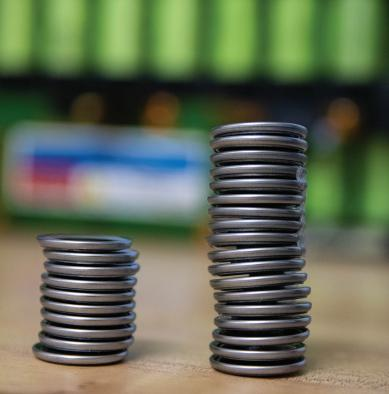
*Top:* Dr. Siu conducts electrochemical tests on potential battery materials. *Bottom:* The lefthand stack of battery cells made of a novel cathode material has the same energy storage capacity as the righthand stack of cells used in the current generation of batteries.
