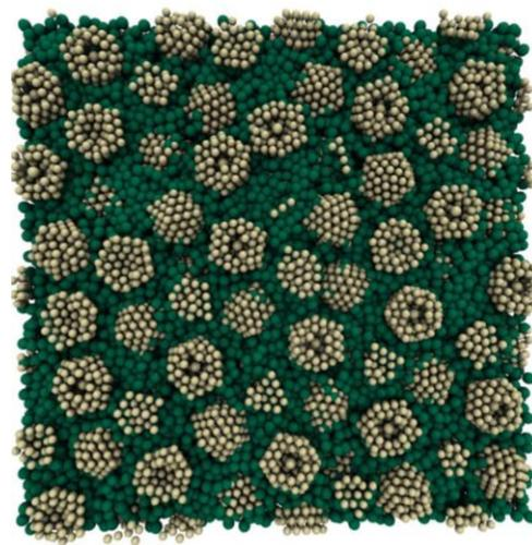
Figure 2. Rendering of a nanocomposite simulation (note all particles are full icosahedra but are visually truncated by the rendering plane). Green beads are polymer segments; gold beads comprise nanoparticles.
