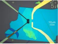
**Figure 3.** A MoTe<sub>2</sub>-based LED and solar cell, built by *Jarillo-Herrero*.
