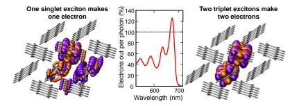
**Figure 1**. Unlike electrons, excitons can be split. In the Center for Excitonics, we have used singlet exciton fission in pentacene to generate at least 1.26 electrons per photon.
