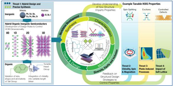
Inorganic/organic components form crystalline HOIS wherein the inorganic component may comprise 0D isolated anions, 1D chains, 2D/quasi-2D planes, or completely interconnected 3D network. CHOISE is uncovering the basic understanding and design rules to uncover unprecedented control over spin, light and charge.
