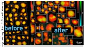
Using sophisticated techniques, EFRC researchers are observing, at the molecular level, how hydrogen fuel cells degrade. Microscope images reveal effects of aging on fuel cell catalyst nanoparticles.
