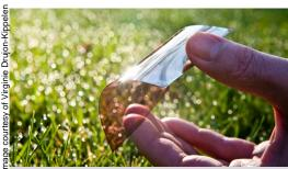
Using polymers to develop new materials, EFRC researchers created the first completely plastic solar cell, where not just the cell itself but also its electrodes are made of plastic.
