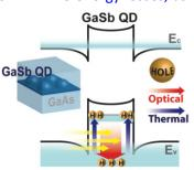
Energy band diagram of a quantum dot with a type II band line-up
