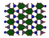
Structure of K<sub>3</sub>Am(PO<sub>4</sub>)<sub>2</sub>
