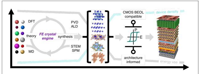
Fig. 1: The 3DFeM vision leverages fundamental understanding of emergent ferroelectricity created via nanoscale inhomogeneity to create memory devices densely interconnected with logic to enable low-power, 3D non-von Neumann computation
