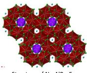
Structure of Na<sub>3</sub>AlPu<sub>6</sub>F<sub>30</sub>
