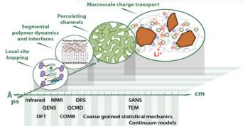
Figure 1 Length and time scales of experiments and theory relevant to the FaCT mission. (QENS = quasielasitc neutron scattering, BDS = broadband dielectric NMR = nuclear magnetic resonance, DFT = density functional theory, DRS = diffuse reflectance spectroscopy, QCMD = quartz crystal microbalance with dissipation monitoring, COMB = charge-optimized many-body potential, SANS = small-angle neutron scattering, and TEM = transmission electron microscopy.)
