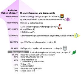
**Figure 2:** Passive (P) and Active radiative (R) systems that become possible with increasingly high optical efficiency.
