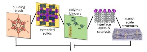
Figure 1: The SCALAR EFRC aims to rethink battery materials, starting from the level of building blocks and then moving to new motifs for extended solids. New materials are integrated with multifunctional polymer binders, designer interfaces, and controlled nanoscale architecture.
