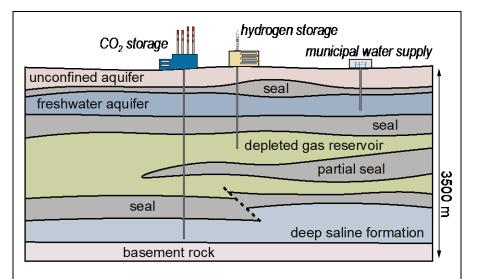
Fig. 1-1. Typical geological strata with seals (unconventional formations). Gas reservoir is repurposed for seasonal  $H_2$  storage. The reservoir seal prevents vertical  $H_2$  movement. Anthropogenic CO<sub>2</sub> is injected into a deep saline formation for secure storage. Top and bottom seals confine CO<sub>2</sub> to the formation.
