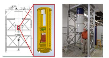
**Fig. 1:** Conceptual layout of a scanning qubit microscope. (left) Dry dilution refrigerator, sensor head, and scanner. (right) Dedicated SQM setup recently installed in the Materials Research Laboratory at the University of Illinois.
