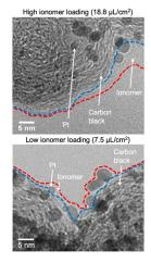
Fig. 2. Non-uniform ionomer distribution revealed by low-dose, cryo-TEM imaging of ionomer-
