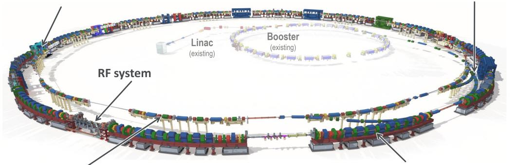
New **accumulator ring** for full-energy swap-out injection and recovery of bunch trains
