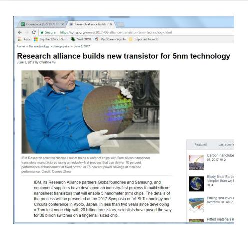
"IBM's said it's using a new type of transistor, called **stacked silicon** nanosheets, to pack transistors this closely together. The nanosheet transistor sends electrons through four gates, as opposed to the current-generation FinFET transistor design that sends electrons through three gates. FinFET (short for fin fieldeffect transistor) began appearing in 22nm and 14nm chips and are expected to continue being used with 7nm chips." June 5, 2017
