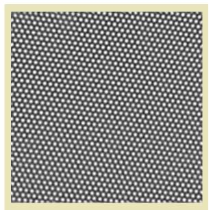
**Fig. A.1. Hexagonal Convection Cells in SF**<sub>6</sub> near **Its Critical Point.** A thin layer of compressed SF<sub>6</sub>, confined between two parallel transparent sheets, is heated from below. The collective behavior of myriad fluid molecules forms a simple convection pattern when the Raleigh number is exceeded. [From G. Ahlers, "Experiments with Rayleigh-Bénard Convection" (www.nls.physics.ucsb.edu/papers/Ah\_Benard\_03. pdf) and from J. Oh and G. Ahlers, unpublished]
