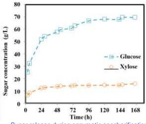
Sugar release during enzymatic saccharification of  $[C_2C_1Im][OAc]$  pretreated switchgrass
