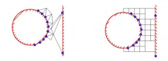
easier grid generation: surface grid not the computational grid (surface description resolves geometry; Cartesian mesh describes flow).
