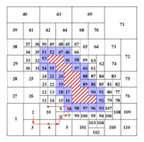
The SFC-ordered mesh puts siblings together, so easy to check if cells can coarsen.
