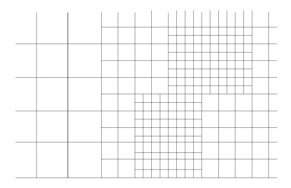
Use recursively nested locally refined block structured grids to attain given level of accuracy.
