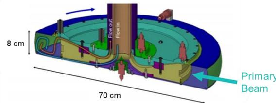
FRIB Beam dump: dissipates the FRIB beam energy and in the process radioisotopes are created in the cooling water.
